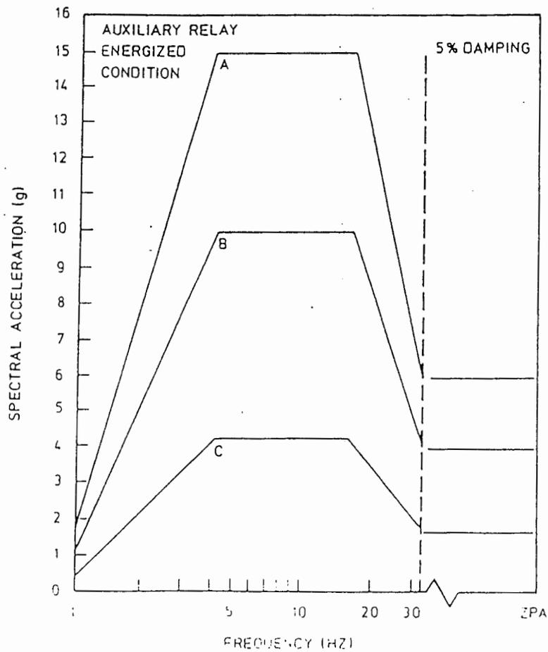
Figure 2-3: GERS for Auxiliary Relays (Energized)
