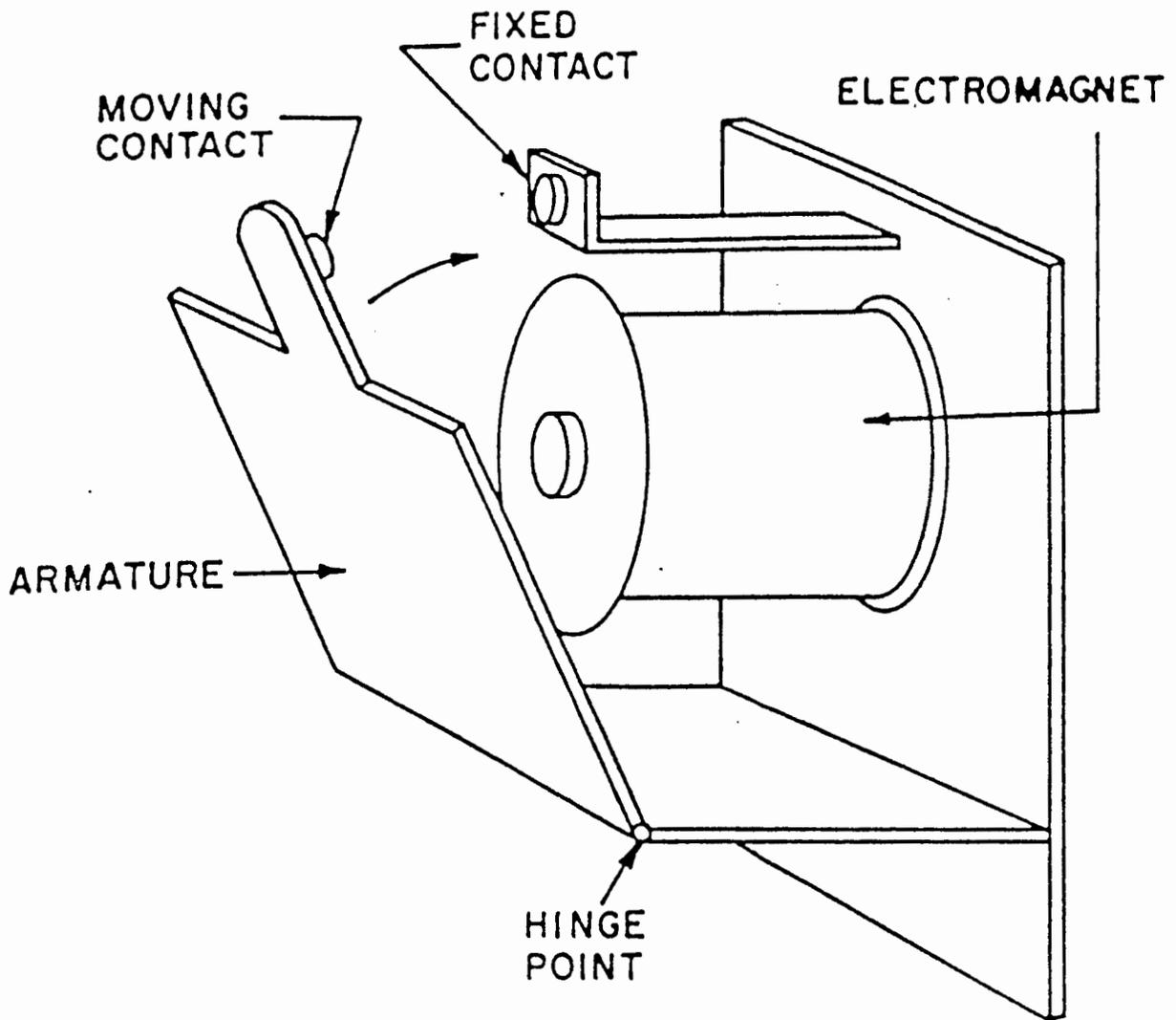
Figure 1-1: Hinged Armature Type Relay Operating Mechanism
