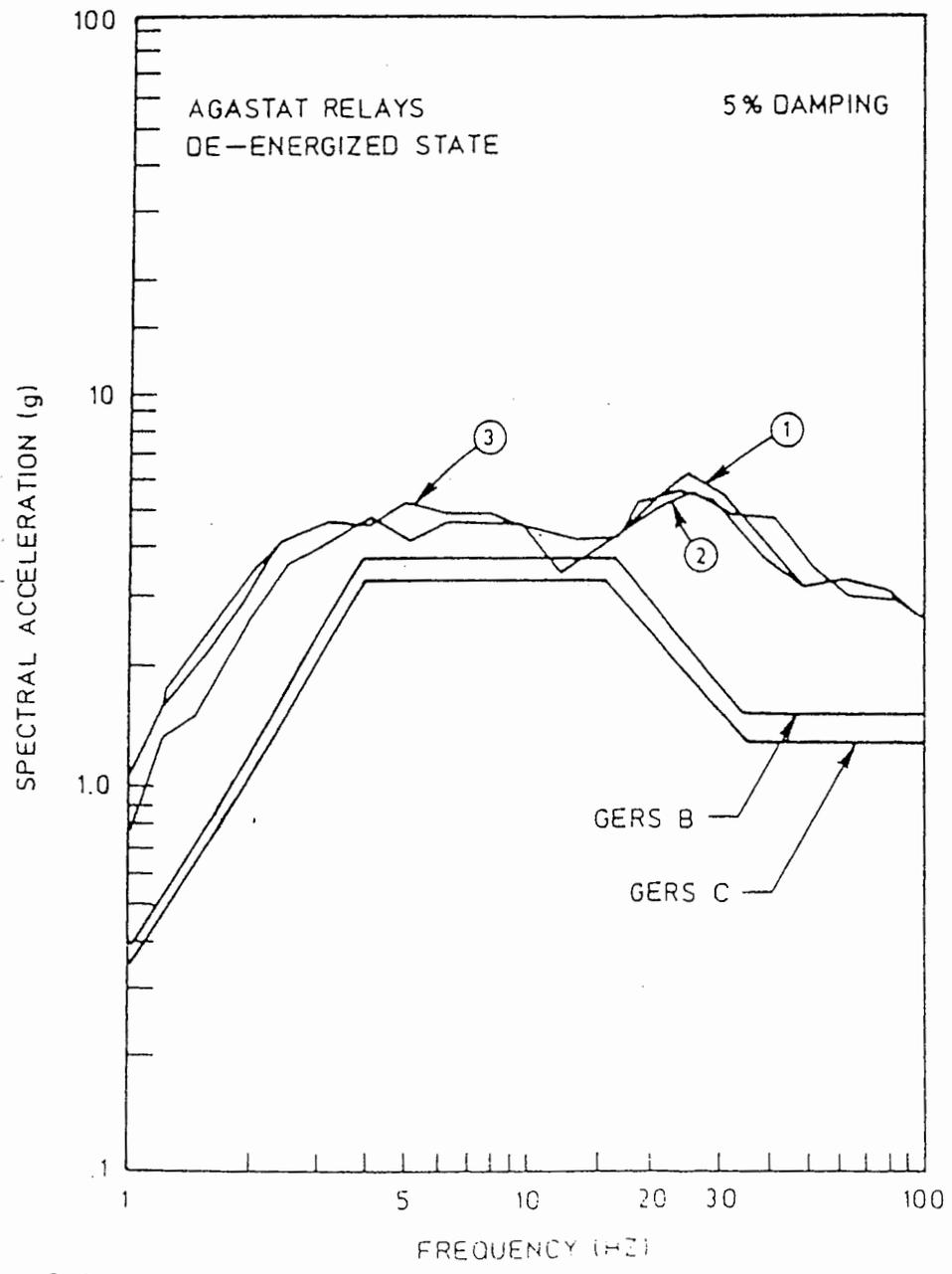
Figure 2-2: Comparison of GERS with Available Fragility Data for Agastat Relays in the De-energized State
