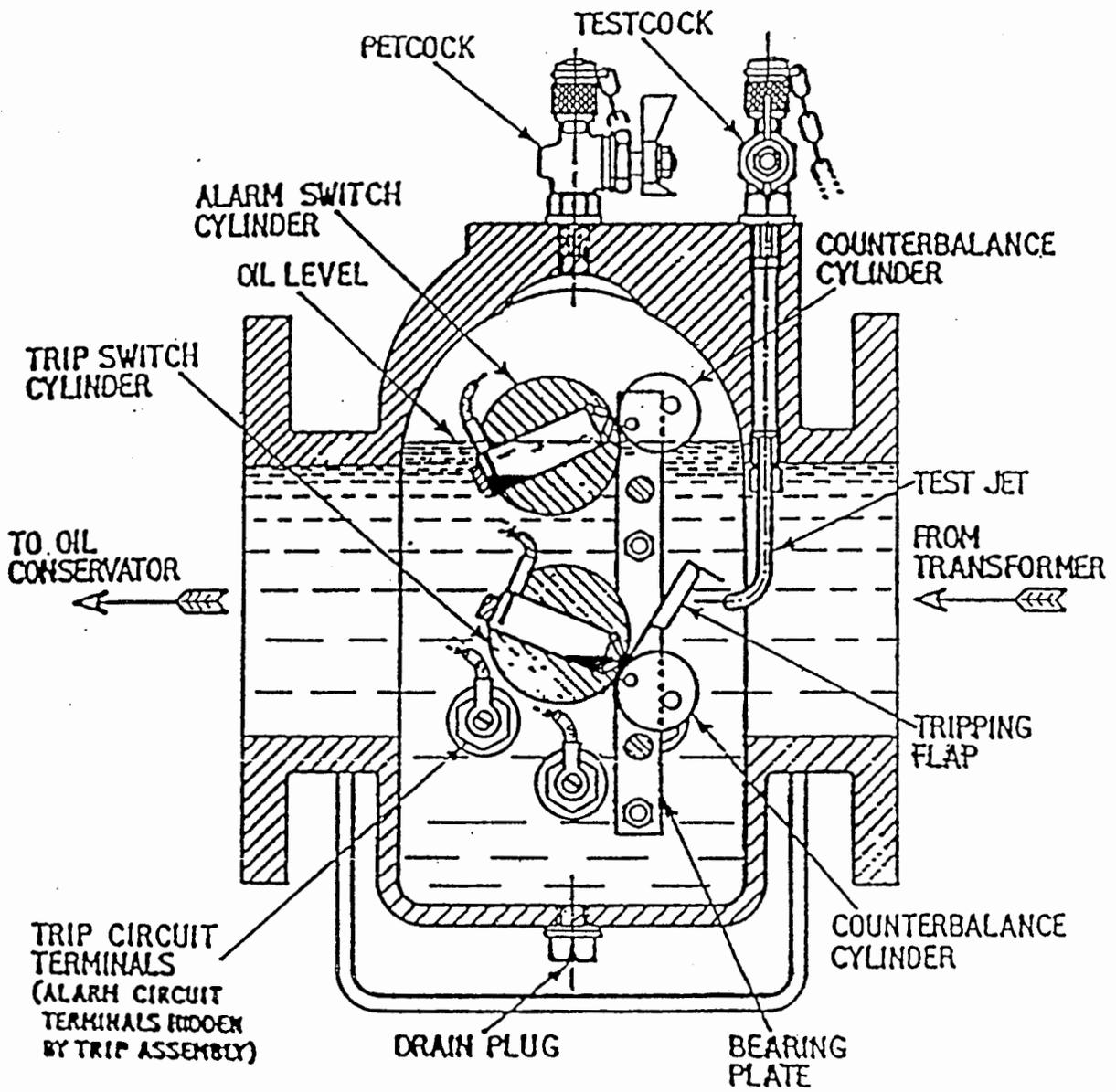
Figure 1-5: Schematic of Sudden Pressure Relay (Buchholz Type)
