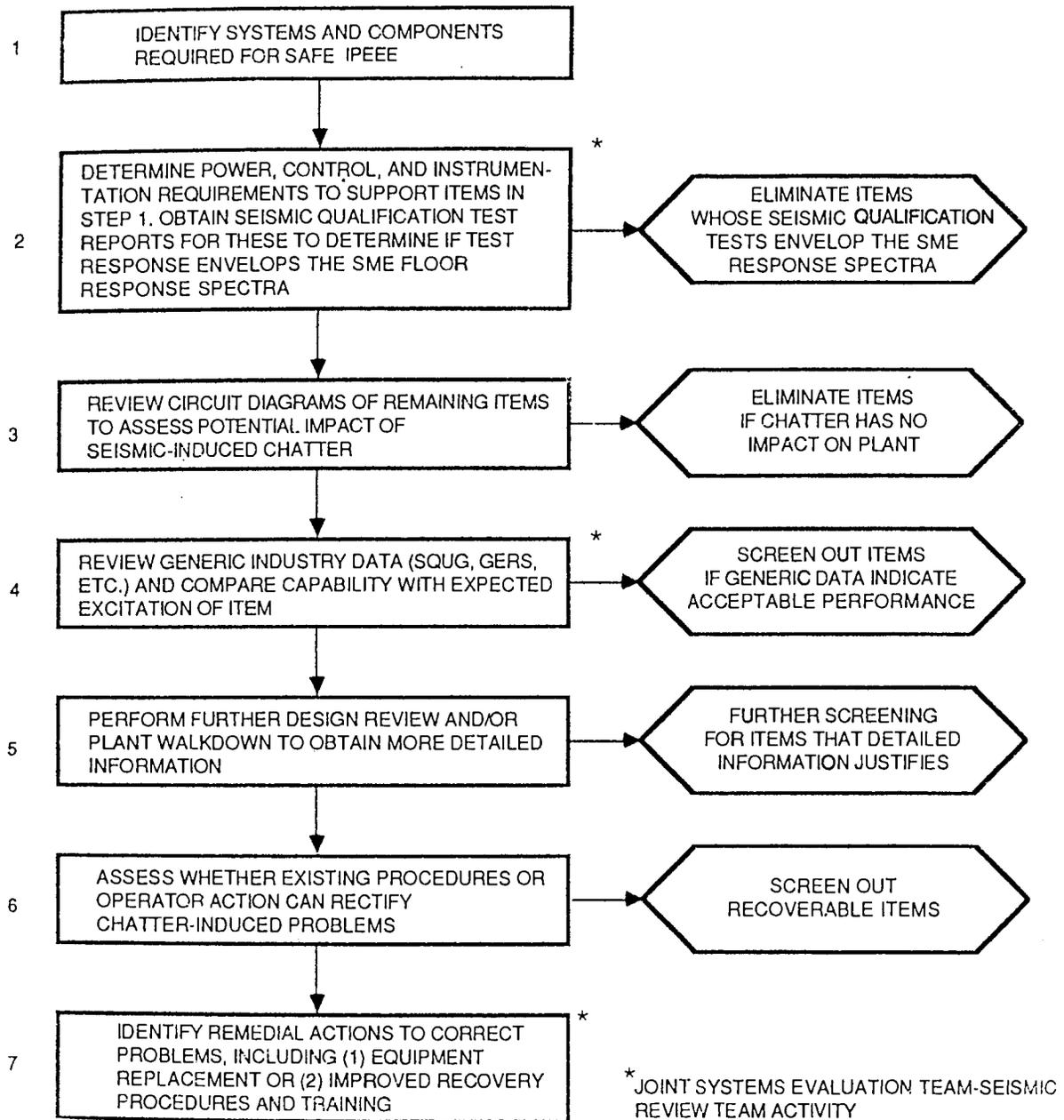
Figure 1-6: Steps in the Assessment of the Potential Effects of Electrical Relay or Contactor Chatter
