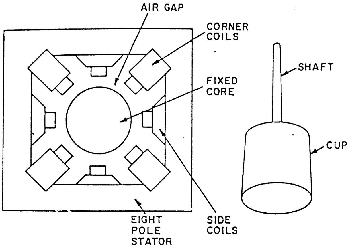
Figure 1-4: Induction Cup Type Relay Operating Mechanism
