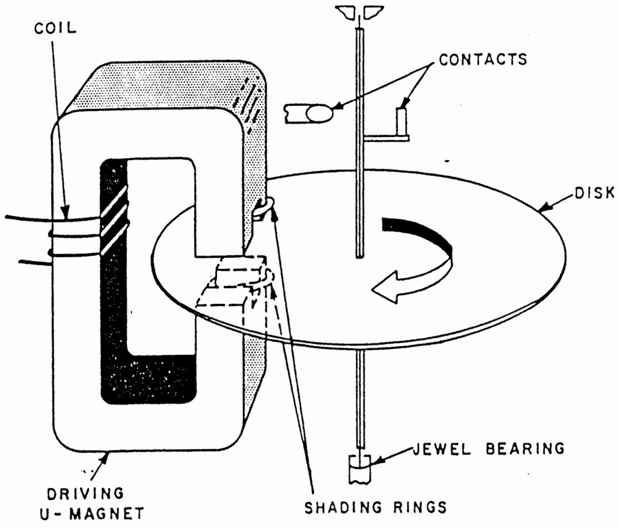
Figure 1-3: Induction Disk Type Relay Operating Mechanism
