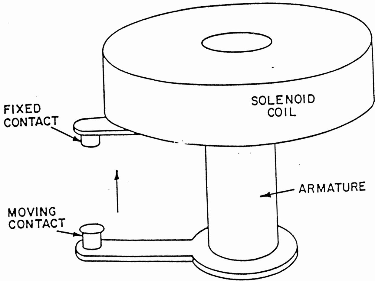
Figure 1-2: Plunger Type Relay Operating Mechanism
