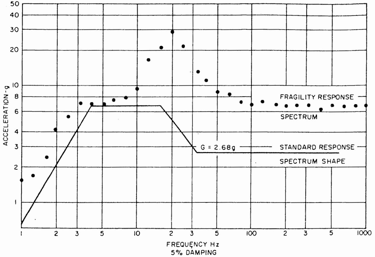
Figure 2-1: Standard Response Spectrum for Relays from ANSI/IEEE C37.98
