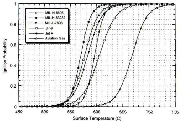
Figure 5 – Ignition Probability as a Function of Surface Temperature for Aviation Fluids, ref (10).
