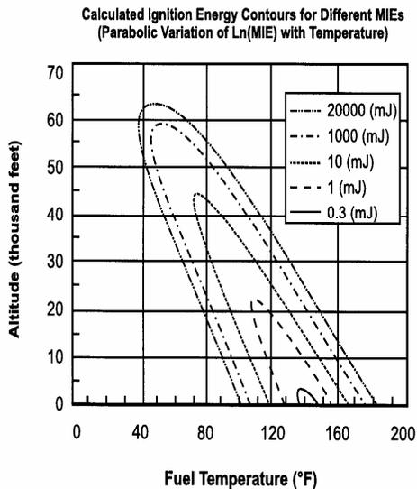
Figure 4 – Constant Ignition Energy Contours Predicted by the Recommended Correlation for a Fuel with a Flash Point of 120°F (49°C) ref (7)
