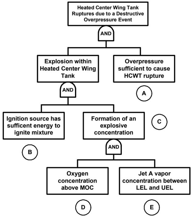
Figure 3 – Generic Fault Tree for HCWT explosion and Rupture
