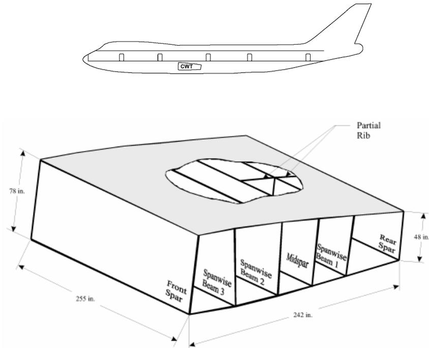
Figure 1. --Schematic of a Central Fuel Tank, Including Dimensions and Partitions, and its Relative Position in a Boeing 747 From a Side View. The Central Fuel Tank, which is also commonly called the Center Wing Tank, is Labeled as “CWT” from Ref. [1] (Modified From NTSB D, 1997 Ref.[2]).
