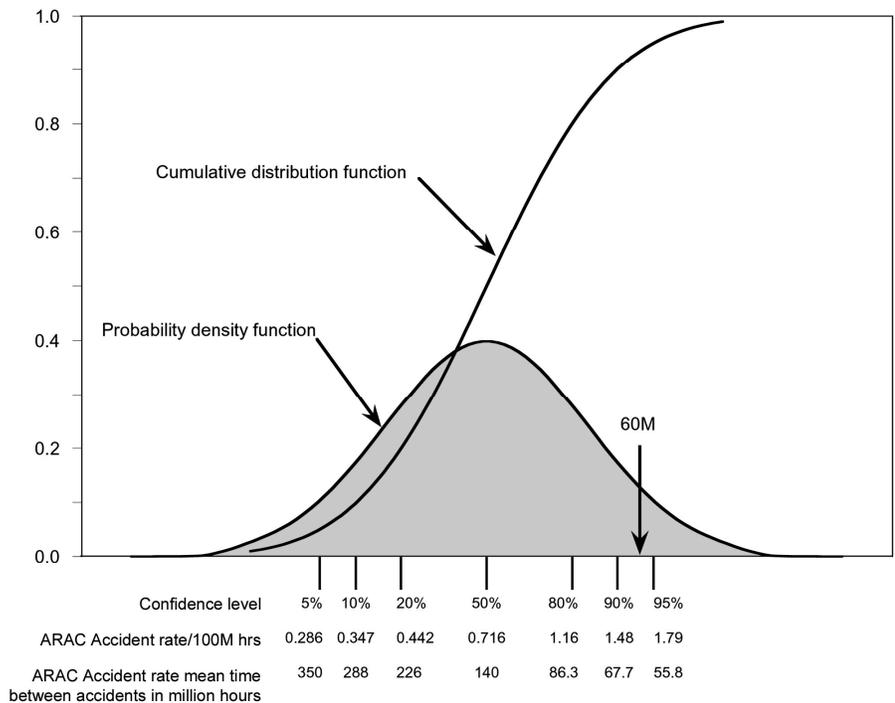
Figure 2 -- Confidence Levels for Catastrophic Heated Center Wing Tank (HCWT) Explosion Rate without SFAR 88 implementation
